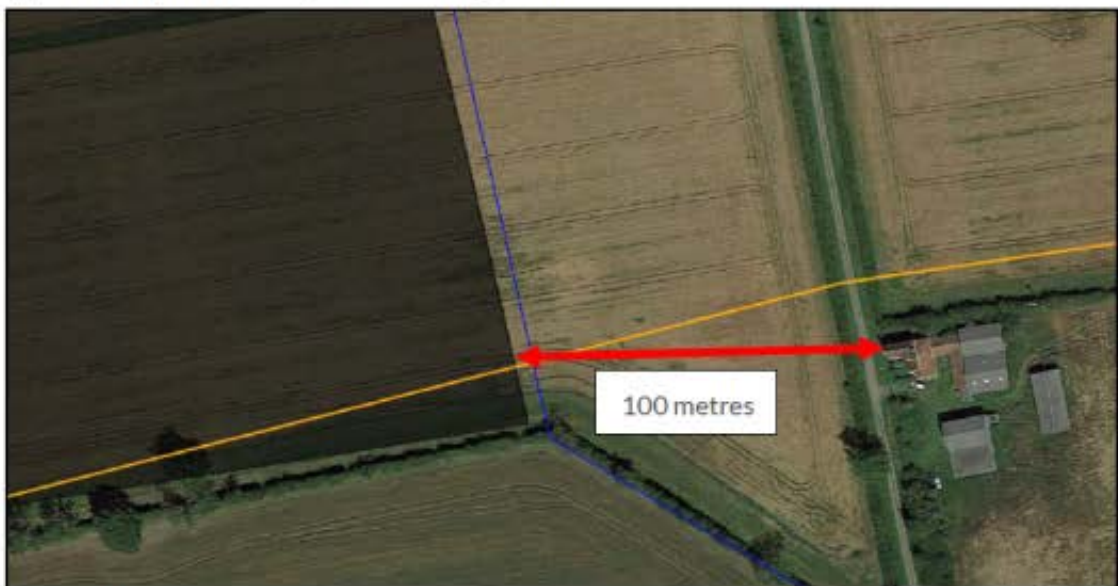
Figure 10 Minimum distance between batteries and a dwelling
